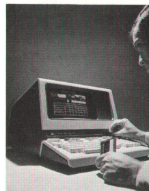
Cover: Model 2644A Terminal is a microprocessor-controlled CRT terminal that has two built-in magnetic tape units for mass data storage. The tape units accept the new 3M Company DC-100 mini-cartridge.
